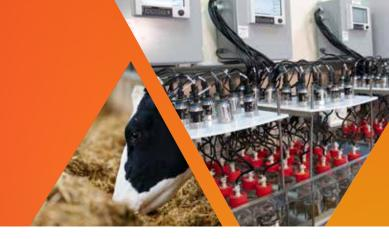
Alltech IFM $^{\text{TM}}$  is an *in vitro* fermentation model that simulates rumen fermentation and evaluates the digestibility of a ration and end-product formation. Alltech IFM is a nutritional tool used by farmers and feed manufacturers to screen individual ingredients, formulate rations and make informed decisions on the quality of feed or total mixed rations (TMR).
